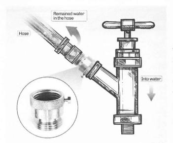
Another method of preventing backflow with a garden hose is using a device known as a vacuum breaker. Vacuum breakers are inexpensive devices that can be screwed onto your outside faucet. These devices will prevent contaminants from being siphoned back into your plumbing and the public water system.
